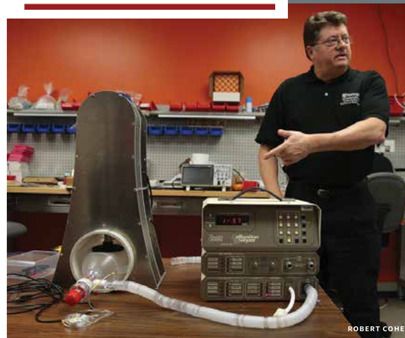
Dennis Mell, an electrical and systems engineering professor at Washington University and chief technology officer at Custom Technologies, talks with his team as he tests a prototype ventilator attached to a calibration machine at Custom Technologies in Brentwood.
