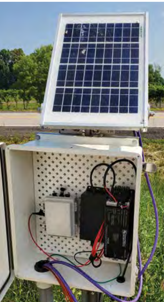
Infratico's roadside unit for collecting test data. PHOTO COURTESY OF INFRATICO
