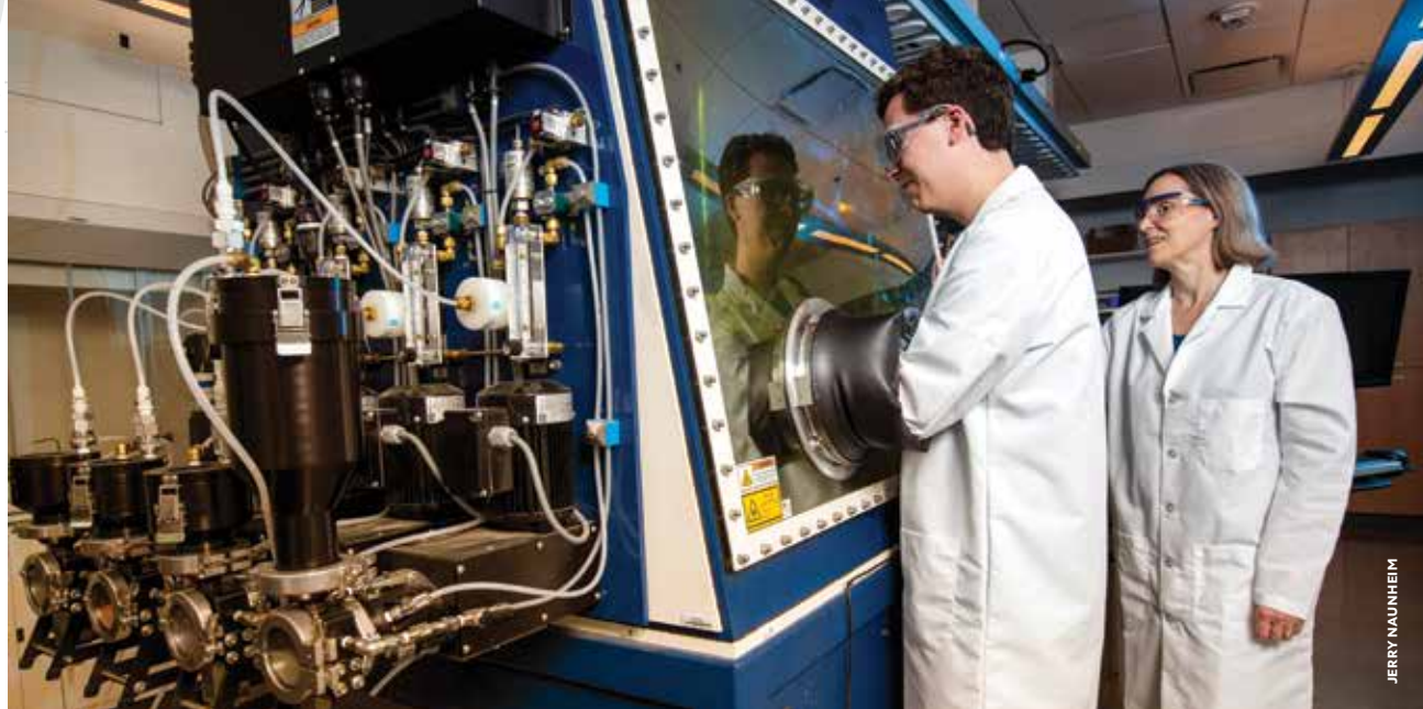
▲ From left: Sam Perkins, a student in the Thermal Management REU program from Bradley University, works with Flores on the Optomec MR-7 Laser Engineered Net Shaping (LENS) system, which is a direct laser deposition system for 3D printing metals.
