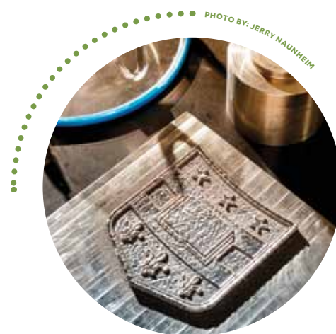
▲ The WashU shield is made from a titanium alloy and was 3D printed using the LENS.
