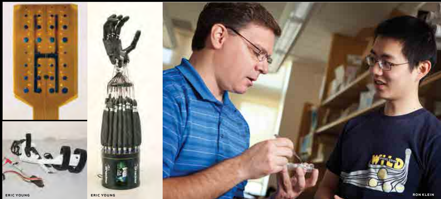
Above, top: A tiny computer chip implanted in the brain records brain activity. Bottom: Brain-controlled hand orthotics can help speed stroke recovery. Center: a robotic arm like this one can be controlled directly by the brain. Right: Dan Moran working with a student in his lab.
