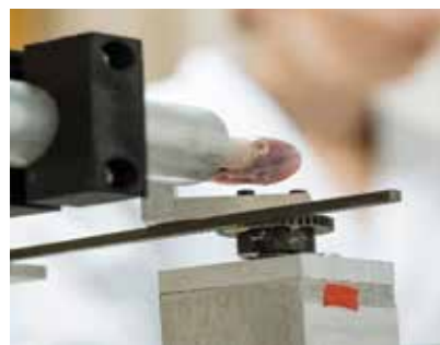
Doctoral student Chelsey Dunham mechanically testing rat elbows in the Lake Lab to evaluate joint motion following injury.
